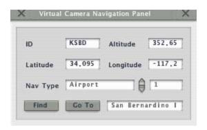
This panel will allow the camera to be located at an Airport, VOR etc. For example set the Nav Type to Airport by using the up/down arrows. Type KSBD into the ID text field and press the Find button. The panel will be updated with the Altitude, Latitude and Longitude. Press the Go To button and the camera will be positioned at that Airport location.
